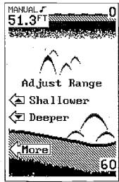
To adjust the upper or lower limit, press the key adjacent to the "More" label. The menus shown below appear. To adjust the upper limit, press the key adjacent to the "Upper Limit" arrow. A new menu appears: "Enter Upper Limit." Using the number keys at the display's left side, enter the desired upper limit. In this example, we used 21 feet. If you make an error, press the CLEAR key and start again. Now press the ENTER key. The X-60 changes the upper limit to the value you entered.
